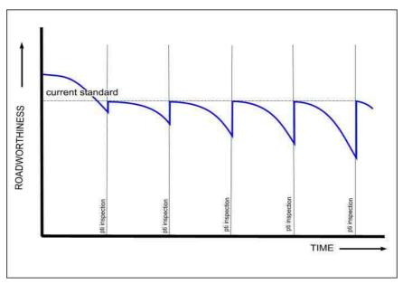
Figure 10: Rate of vehicle deterioration
