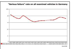
*Figure 4: Failure rate of 3 million passenger cars in Germany.*
