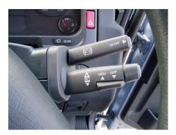
Figure 27: MAN TGL cruise control column stalk
