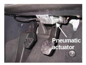
Figure 3: ISA brake actuator
