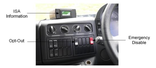
Figure 29: HMI in the ISA truck
